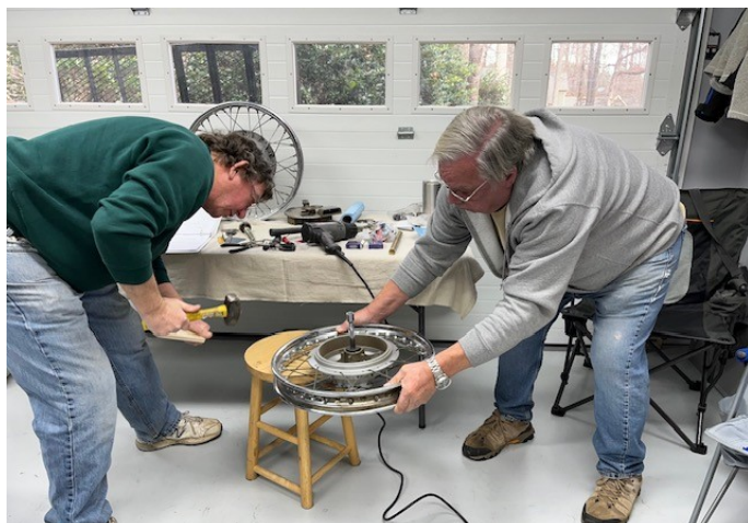
Installing New Wheel Bearings
