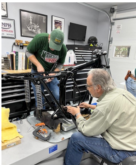
Installing swing arm with new bushes
