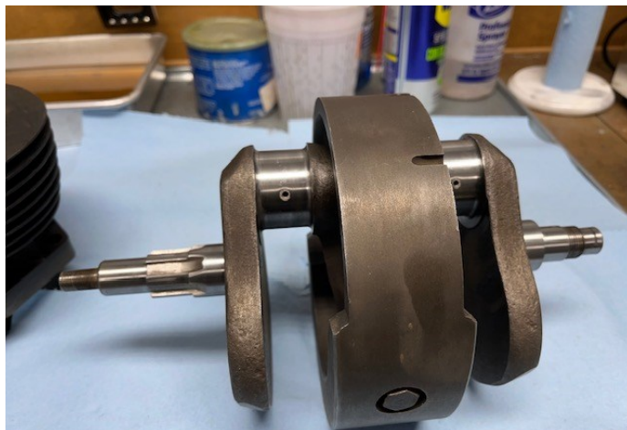
Crankshaft polished—New sludge trap installed
