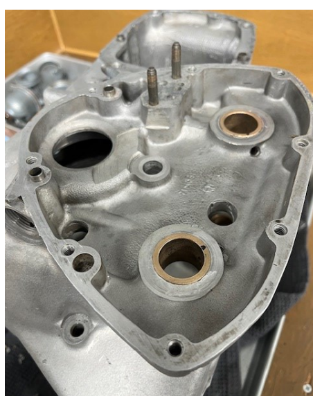
New Cam Bushes installed and reamed
