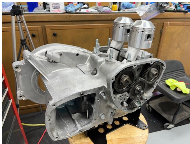
Cases Installed and timing set
