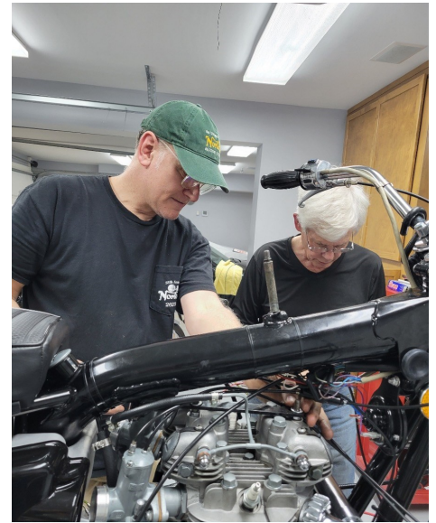
Installing rocker boxes
