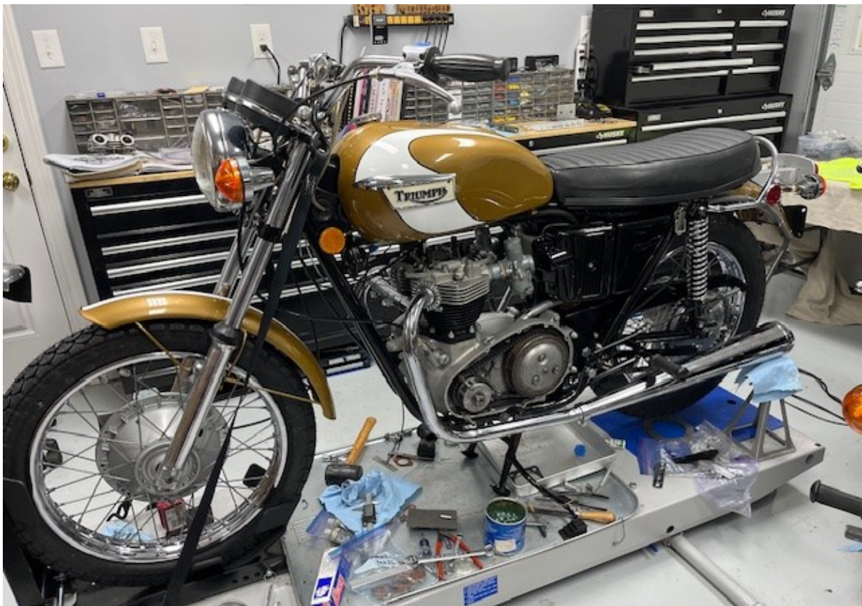
Carbs and exhaust Installed
