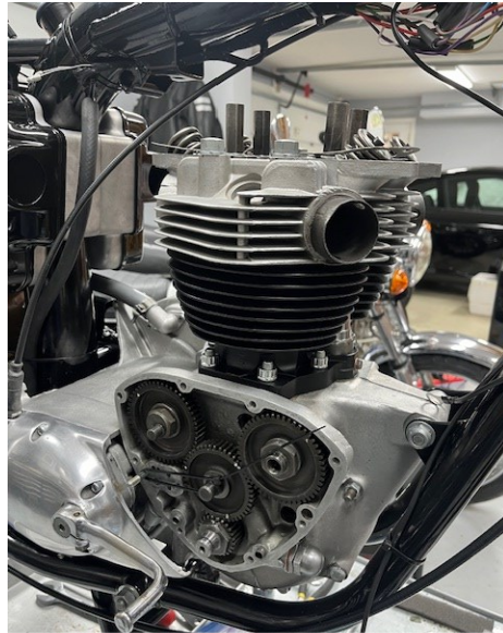
Cylinder head installed
