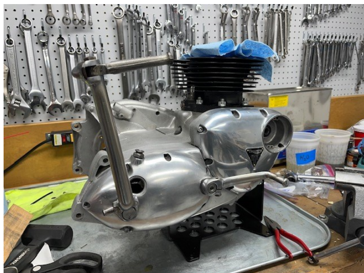
Gear Box installed
